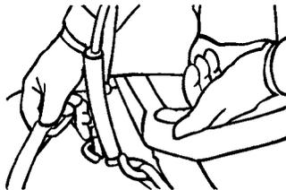
Secure the front of the scooter by hooking each belt to the tiller and crisscrossing them in front.
