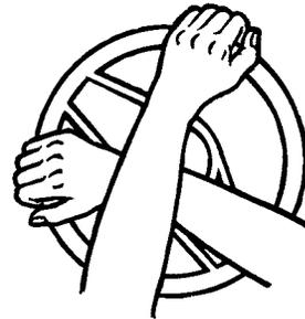
During a turn, the hand-over-hand steering method is the best to use. One hand pushes the steering wheel up, across and down, while the other hand reaches up to the top of the wheel and pulls down. This action is repeated grasping the wheel at the top again.
